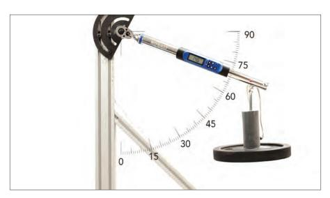
Students overlay tools onto high-quality videos to make measurements, such as in this activity where torque is calculated.
