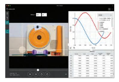
Show the link between circular motion and simple harmonic motion.
